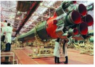
are then discarded. The separation time is determined by comparing the velocity with a predefined value. Thrust is transferred through a ball joint located at the top of the cone-shaped structure of the booster, which is attached to the central core by two rear struts.
