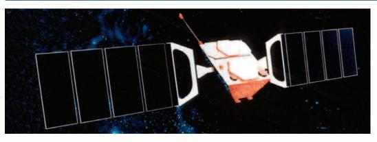
Each first-generation Globalstar satellite, designed by Space Systems/Loral, is a three-axis stabilized spacecraft consisting of a trapezoidal main body, two solar arrays, and a boom-mounted magnetometer. Mass of the satellite is approximately 450 kilograms.
